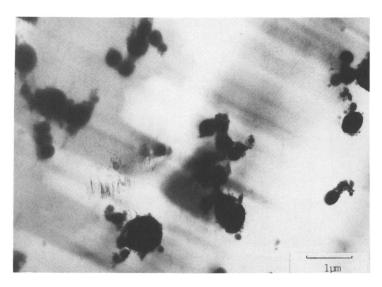
Figure 5. TEM micrograph of 5 phr MG50A-BADGE-pip.
