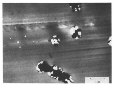
Figure 3. TEM micrograph of 2.9 phr PMM-2.1 phr MG30-BADGE-pip, showing the effect of excess PMM.
