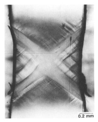
Figure 5. Polarized optical micrograph of the yield zone of 1.20-mm-thick PC loaded to 58.5 MPa and viewed in the yz plane (1).
