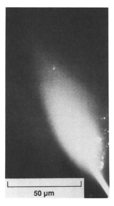
Figure 29. SEM micrograph of the deformation zone in NR-150B<sub>2</sub>.
