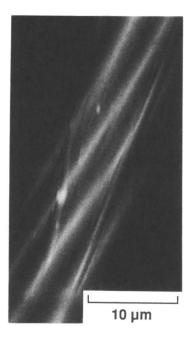
Figure 22. SEM micrographs of the deformation zone showing shear bands in New TPI.
